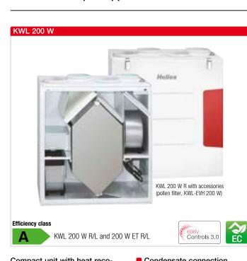
Compact unit with heat recovery for the central supply and extract ventilation of residential buildings and apartments. Perfectly prepared for modern communication and operation with the new Helios easyControls 3.0 control system incl. integrated network connection. Equipped with EC fans for low energy consumption and highly efficient plastic or enthalpy heat exchangers for additional moisture recovery.
